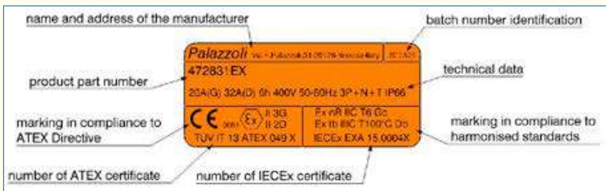
Picture 30: label example of a Palazzoli ATEX interlocked socket
